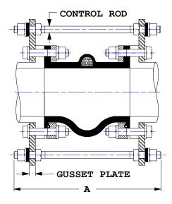
The flexible rubber sleeves of expansion joints, filled arch or open arch construction must be installed in piping systems that are properly anchored so that the flexible sleeves may not be subjected to compression or elongation of piping movement.
